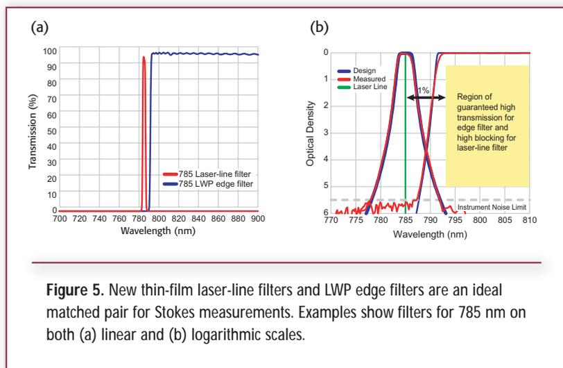
**Figure 5.** New thin-film laser-line filters and LWP edge filters are an ideal matched pair for Stokes measurements. Examples show filters for 785 nm on both (a) linear and (b) logarithmic scales.
