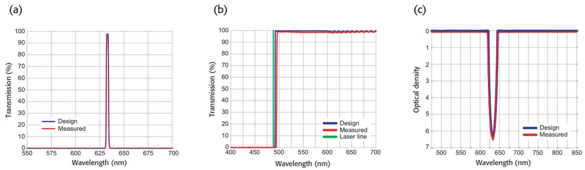
**Figure 3.** Spectra of modern thin-film filters, showing both target design and typical measured example spectrum: (a) 632.8-nm laser-line filter; (b) 488.0-nm LWP edge filter; and (c) 632.8-nm notch filter.
