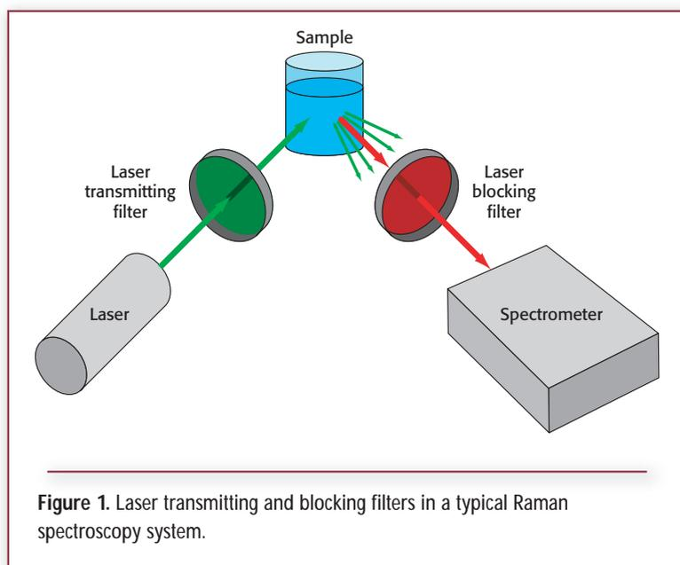
**Figure 1.** Laser transmitting and blocking filters in a typical Raman spectroscopy system.
