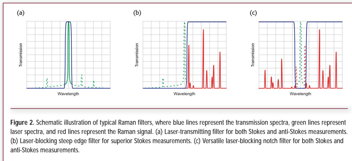
**Figure 2.** Schematic illustration of typical Raman filters, where blue lines represent the transmission spectra, green lines represent laser spectra, and red lines represent the Raman signal. (a) Laser-transmitting filter for both Stokes and anti-Stokes measurements. (b) Laser-blocking steep edge filter for superior Stokes measurements. (c) Versatile laser-blocking notch filter for both Stokes and anti-Stokes measurements.
