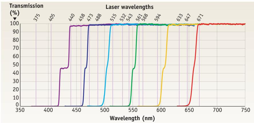
**FIGURE 4.** Systems with multiple lasers for exciting a variety of fluorophores require the lasers to be combined together efficiently. Dichroic beamsplitters of 45° allow highly efficient laser-beam combining (nearly 100% reflection and transmission) and are optimally matched to the most popular laser lines used in fluorescence imaging.
