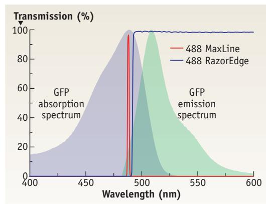
**FIGURE 1.** A narrow laser line combined with a narrowband laser-line cleanup filter allows optimal excitation of the desired fluorophore (here green fluorescent protein, or GFP). This, combined with a steep edge filter allows almost perfect spectral efficiency for collection of weak fluorescence signals.
