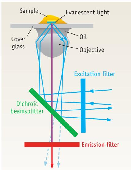
**FIGURE 2.** Different configurations of the excitation light path can be used to create TIRF excitation. In this configuration, the sample is illuminated through a high-numerical-aperture objective (NA of approximately 1.45).
