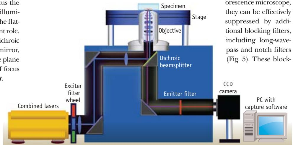
**FIGURE 3.** An inverted microscope configuration for TIRF illumination includes a focusing lens, mirrors, and a detector such as a computer-controlled CCD camera. To suppress the reflected excitation light that “leaks” past the dichroic beamsplitter in the emission channel, often an additional blocking filter is used in combination with an emission filter.
